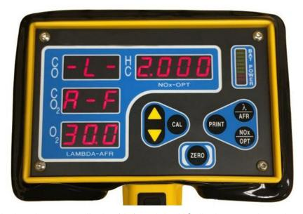
The CO display changes to display '-L-', and the HC display now shows Lambda to 3 decimal places as X.XXX. The  $CO_2$  display changes to read 'A-F' and the  $O_2$  display now shows real-time A/F ratio. NOTE: Both Lambda and A/F ratio are calculated from exhaust gas readings, and use the selected fuel constants to complete the calculation. See White Paper #1 - Lambda Calculation – The Brettschneider Equation, general principles and methods for more information about Lambda.
