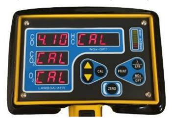
9. When the CO gas is calibrated, press the CAL button to select the next gas to be calibrated. In this illustration, the HC channel shows it is ready for span calibration. Use the UP and DOWN arrow buttons to adjust the gas concentration reading to match the calibration gas tag value. Note: Your analyzer automatically changes its HC channel to match the HC in calibration gas cylinders. It changes back on CAL mode exit.
