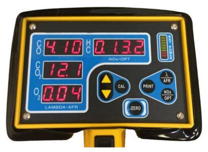
Pressing the " $NO_x$  / OPT" button again changes the HC display back to the normal measuring mode for the selected fuel.
