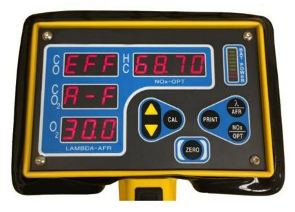
Pressing the UP arrow changes the CO display to read 'EFF', and the HC display now shows Combustion Efficiency % to 2 decimal places as YY.YY. NOTE: Combustion Efficiency is a measure of the efficiency of the engine to burn fuel, and is calculated from the exhaust gas readings using fuel – specific constants.
