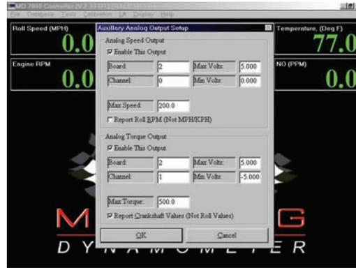
Since some dynamometer users use external data acquisition systems, your system can be configured to drive two (2) analog outputs proportional to the speed and torque measured by your dynamometer. These outputs can be fed to the analog inputs of a data acquisition system.
