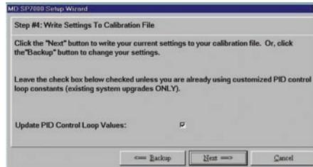
This page allows the operator to specify whether PID control loop values should be updated (normally yes), and writes the new values to the application's Ini file.
