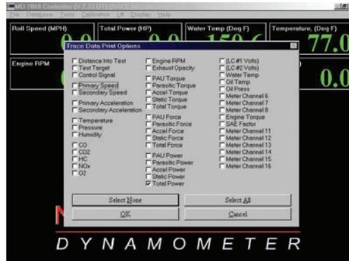
Notice that the channels displayed on this form represent the left-mouse-button and right-mouse-button menus that can be used to select value for display on the main screen.
