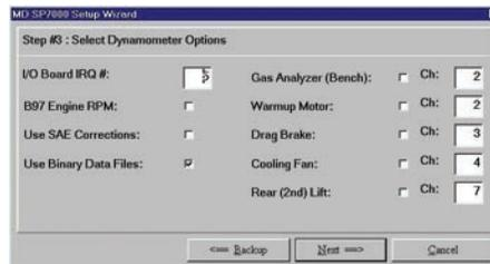
This page allows the operator to review and/or modify several dynamometer option values.
