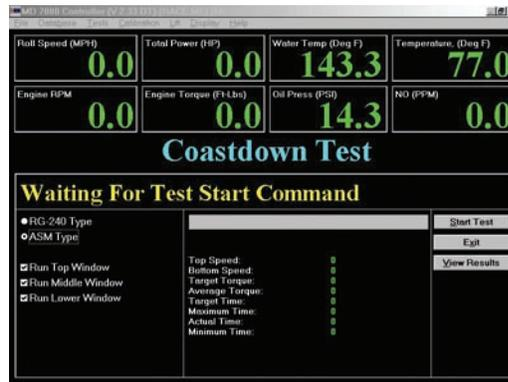
This test is used to perform an automatic coast-down verification test. Coast-down tests are used to verify that the dynamometer is properly calibrated by decelerating the dynamometer's inertia using the dynamometer's PAU. The time required to decelerate a known mass by a known amount using a known force can be calculated, and the actual time required is compared against the calculated time.
