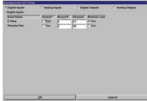
This view of this screen allows the operator to specify the I/O channels used by the dynamometer control system for digital inputs.
