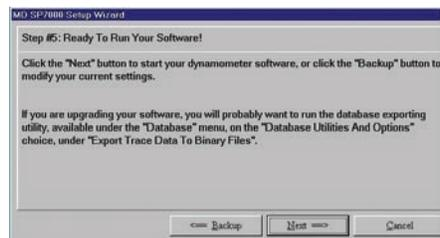
This page allows the user to confirm that the current settings are correct, and launch the dynamometer control software.
