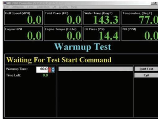
This test is used to bring the dynamometer's bearings, belts, etc. up to a warmed up condition.
