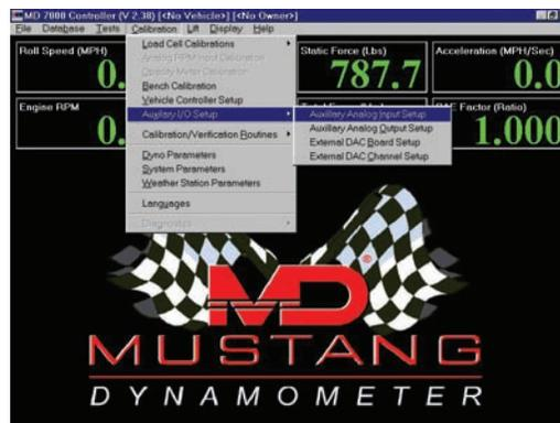
The "Auxiliary Analog Input Setup" menu item allows access to the setup screen used to configure the auxiliary analog inputs used for extra data acquisition hardware, e.g. exhaust gas oxygen sensors, pressure sensors, etc.
