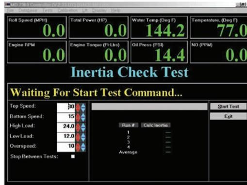
This test is used to measure the inertia (actually, vehicle-equivalent weight) or the dynamometer. This test is used in manufacturing and test-out at Mustang Dynamometer, and is not normally used in the field, unless mechanical changes are made to the dynamometer.
