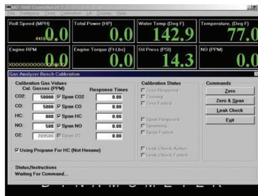
The optional Andros 5-gas analyzer bench supports 3 fully automated self-calibration routines, using ambient atmospheric air for zeroing and a 4-gas blend in a calibration gas bottle for spanning.
