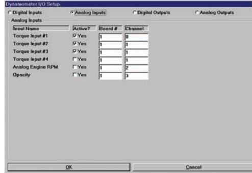
This view of this screen allows the operator to specify the I/O channels used by the dynamometer control system for analog inputs.
