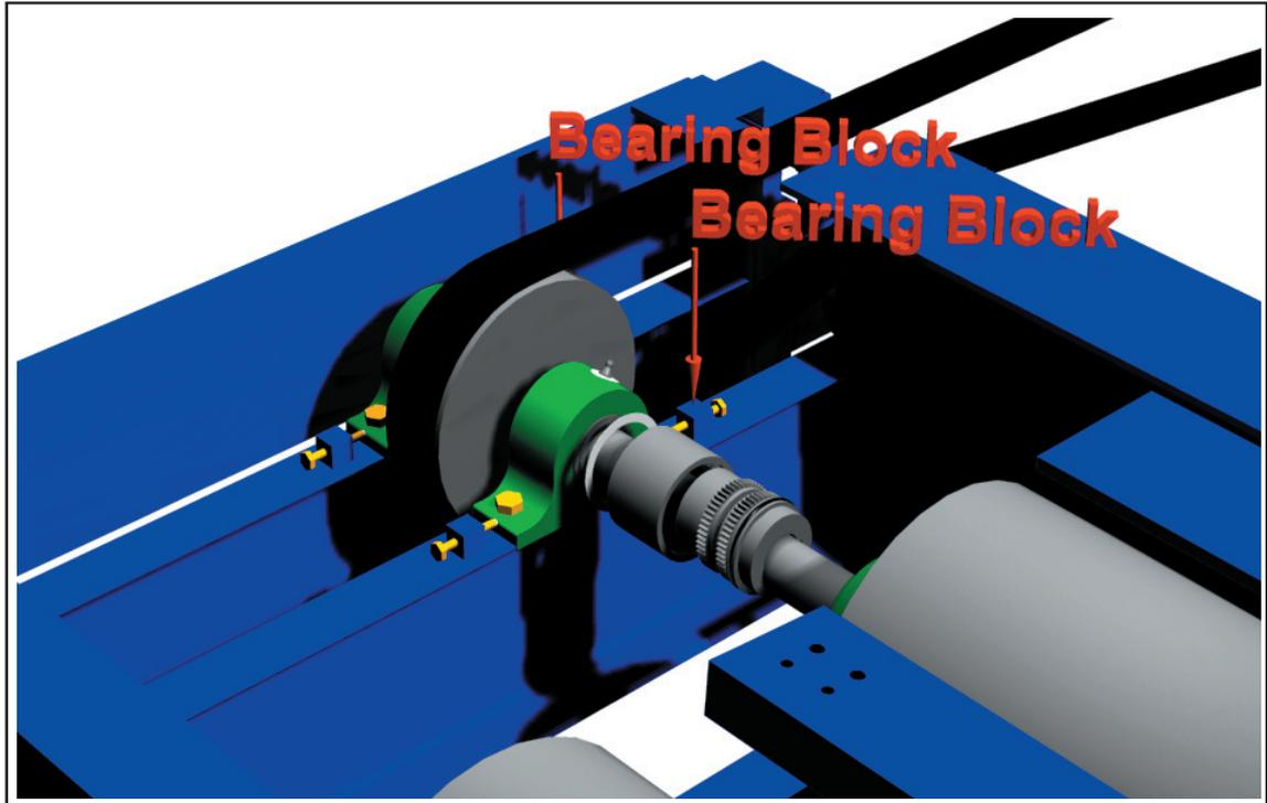
Move these bearing block bolts only. The other two are set in place for alignment.
