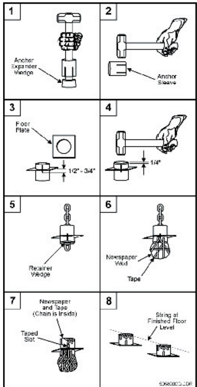
**CAUTION:** Allow the new concrete floor to cure for 11 weeks before pulling on the anchors. The newspaper wrapped under the anchor will decompose, leaving access for chain removal
