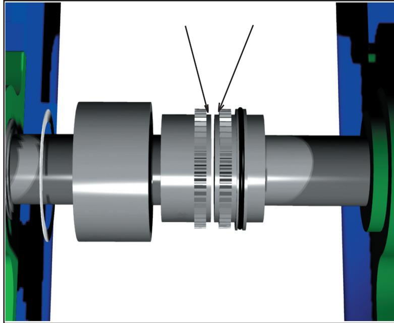
"Face to face" gap should be .125. Use this ledge to check top-bottom and side to side alignment.
