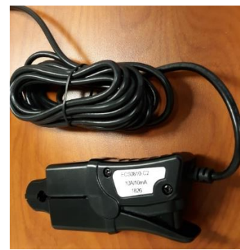
CT Probe: Only compatible when used with the JB Tach Adaptor unit.
