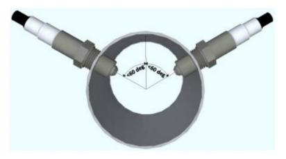
For all Oxygen sensor installations the sensor must be installed before the catalytic converter. For normally aspirated engines the sensor should be installed about 2ft from the engine exhaust port. For Turbocharged engines the sensor should be installed after the turbocharger. For Supercharged engines the sensor should be installed after the turbocharger.
