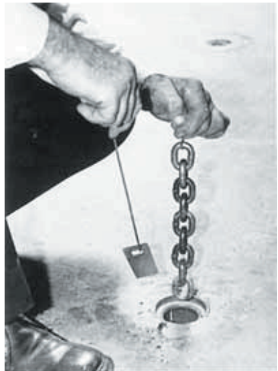
Work chain loose from anchor expander and adjust to desired height. Replace retaining wedge when finished.
