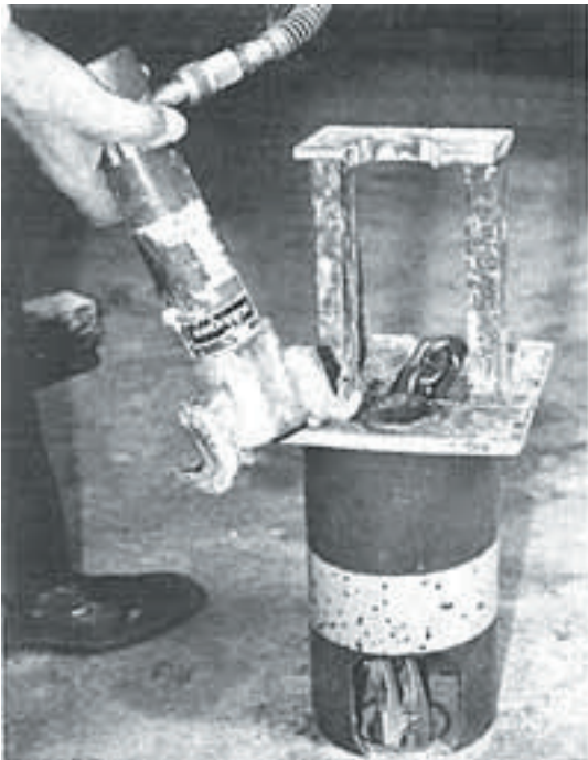
Install ram and puller claw assembly into press if not already prepared.
