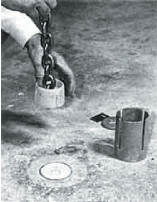
Insert chain retaining wedge and press firmly into slot. DO NOT ATTEMPT TO PRESS WITHOUT RETAINING WEDGE!
