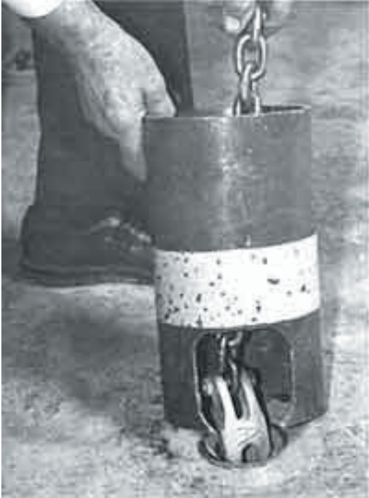
Position remover tube over anchor as shown with puller claw and chain.
