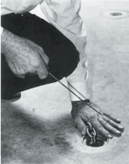
Use a length of welding rod with hooked end (or similar tool) as a means to hook into retaining wedge slot.
