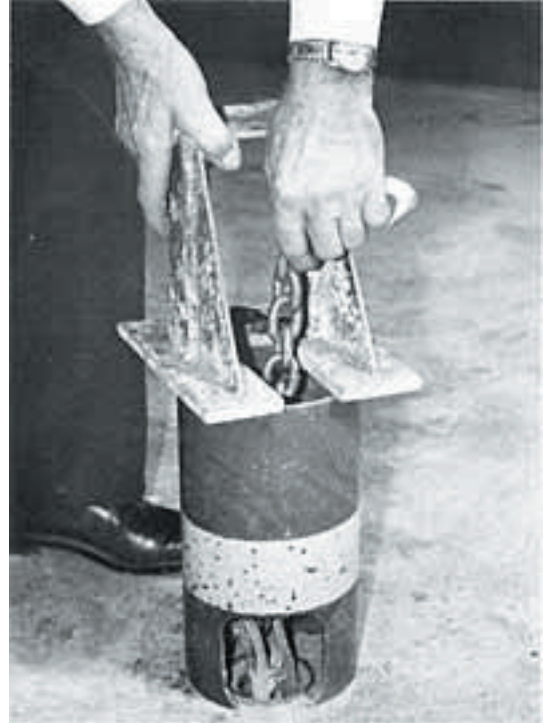
Position anchor press over puller tube as shown with chain protruding from opening.
