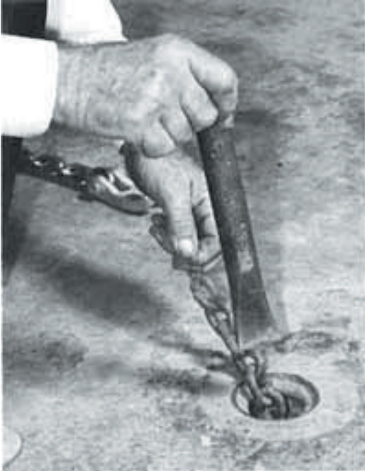
Pull chain aside to make room for blunt instrument to be used as a driver.
