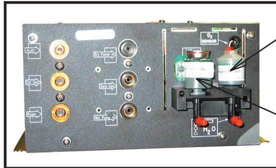
To remove the O<sub>2</sub> Sensor unplug wires going into the top and turn counter-clockwise
