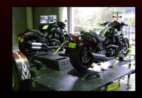
SIDE-BY-SIDE MOTORCYCLE DRAG RACING. Twin MDC-325 Motorcycle dynos for side-by-side racing excitemement.
