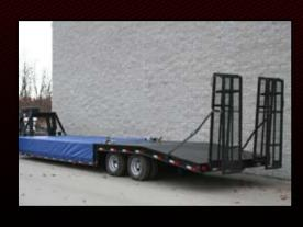
**PORTABLE MD-AWD-500.** Mechanically-linked AWD performance dynamometer. Tightly-engineered to squeeze into a mobile trailer so you can take the show on the road.
