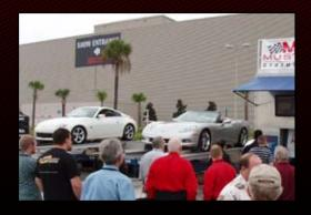
**PORTABLE SIDE-BY-SIDE DRAG RACING DYNOS.** Trailer-mounted side-by-side 2WD performance dynamometers - a virtual race track on wheels.
