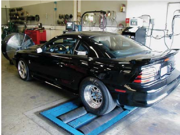
With a 600-hp PAU, the MD-250 is ideal for testing mid-sized trucks and high-performance street cars.
